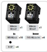
12 Assemble **DYNAMIXEL(ID 13)** to **FR12-H101K** using **WB-M2x3**
